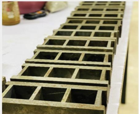
**Mortar and Concrete Molds**
