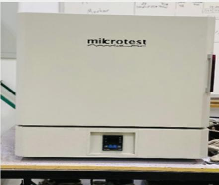
**Muffle Furnace (1200 C)**
